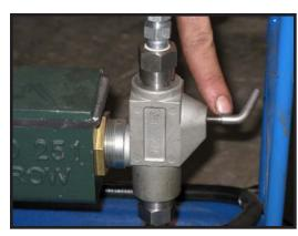
periodic check to see that oil is being injected. Open the port ½ turn while pump is cycling. Allow pump to cycle until oil appears.
